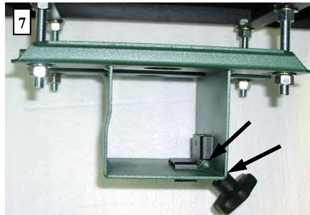
Pallet Corner Clamping Knob Thread Lubricant (lubricate threads and contact point stud to Corner Washer)
